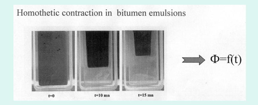
Once the droplet charge is destroyed the droplets are strongly attracted to one another. The asphalt will coagulate even with water still present.
